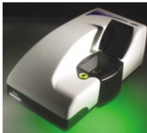
Figure 5 The Zetasizer Nano, a combined static, dynamic, and electrophoretic light scattering system.
