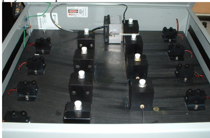
Figure 1. A photograph of the open SMSLS. Shown are the eight lasers, and the eight sample cells. 3 mL sample cells are placed in the cell holders. One cell shows the peltier/fan attachment that allows for cooling.
